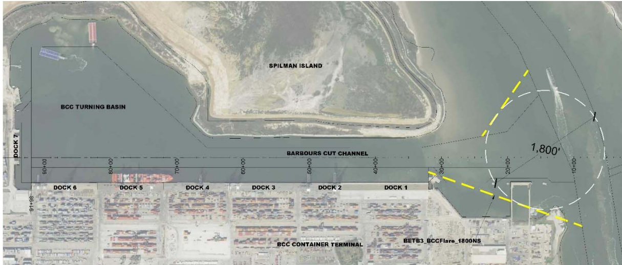
Figure 4-3: BETB3_BCCFlare_1800NS – BCC Flare Easing and 1,800-Foot Turning Basin
