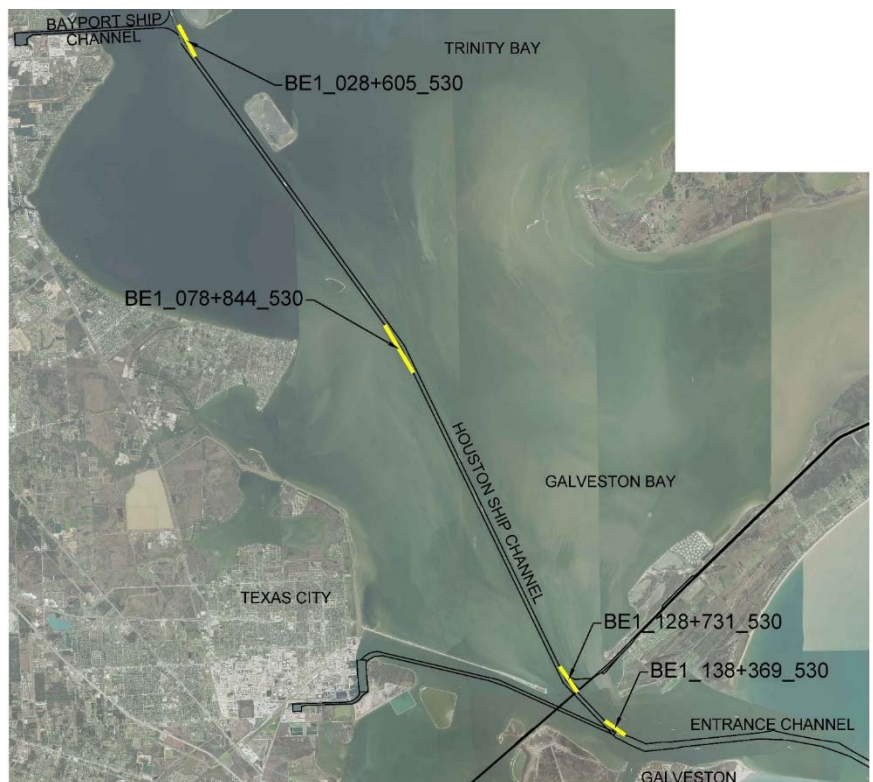
Figure 4-1: Segment 1 Bay Reach Bend Easing Measures for the Existing 530-foot channel
